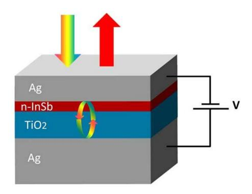
Schematic structure of an electrically tunable perfect light absorber.
