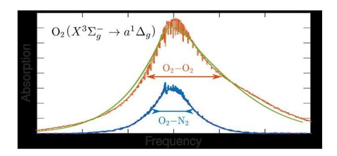
Figure: Experimental and theoretical spectra for light absorption due to the collision of oxygen (O2) molecules with other oxygen molecules and with nitrogen (N2) molecules. As shown here, the absorption due to O2 -O2 collisions is much stronger than due to O2-N2 collisions and the line is much wider than in the first case. Credit: Radboud University
