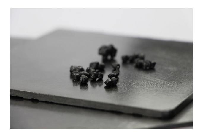
The Fraunhofer ICT uses recycled, small chopped carbon fibers (top) to produce bipolar plates (bottom) for batteries and fuel cells. Credit: Fraunhofer ICT
