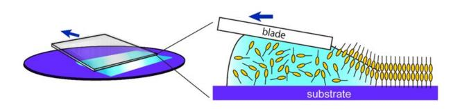
Artist's representation of the blade coating solution process to produce single molecular bilayer thin film transistors. Liquid molecules are spread by a blade over the production surface at room temperature and standard air pressure in a technique called solution processing. As the liquid dries, the inter-molecular forces cause the molecules to automatically arrange themselves into geometrically frustrated single bilayers just 4.4 nanometers thick. Credit: Shunto Arai and Tatsuo Hasegawa
