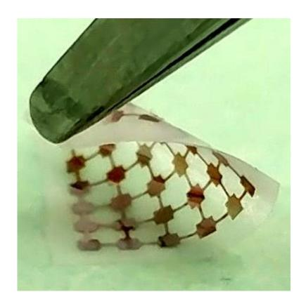
A flexible silicon mesh can adapt to the soft surface of the brain for stimulating neural activity. Credit: Jiang et al/University of Chicago
