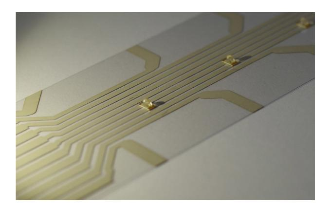
The Fraunhofer ENAS manufactures printed circuit boards in screen printing on a flexible plastic film. The tracks transmit electrical impulses – for example, to make LEDs glow. Credit: Fraunhofer ENAS
