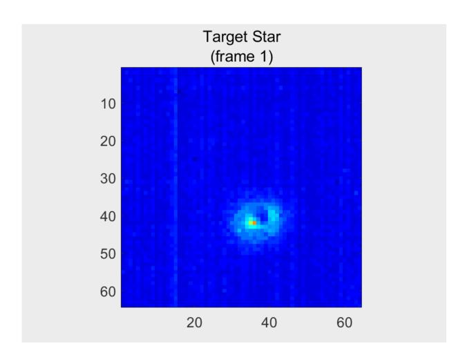
This gif shows a series of images from a single observation of a star by the ASTERIA spacecraft. In the first few images, the star appears to move as ASTERIA slews to and then locks onto the target star. Throughout the remainder of the frames, the spacecraft remains locked on the target star. Credit: NASA/JPL-Caltech
