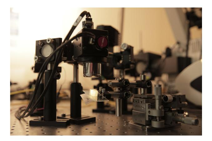
This custom-built optical coherence tomography instrument uses visible light to view tissue. Credit: Renee Meiller
