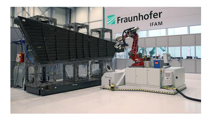
The mobile robot is processing the tail-fin of an Airbus 320 aircraft. Credit: Fraunhofer IFAM
