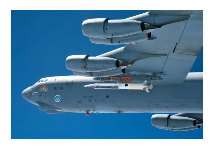
This 2010 US Air Force file photo shows an X-51A WaveRider hypersonic flight test vehicle under the wing of a B-52 Stratofortress during testing
