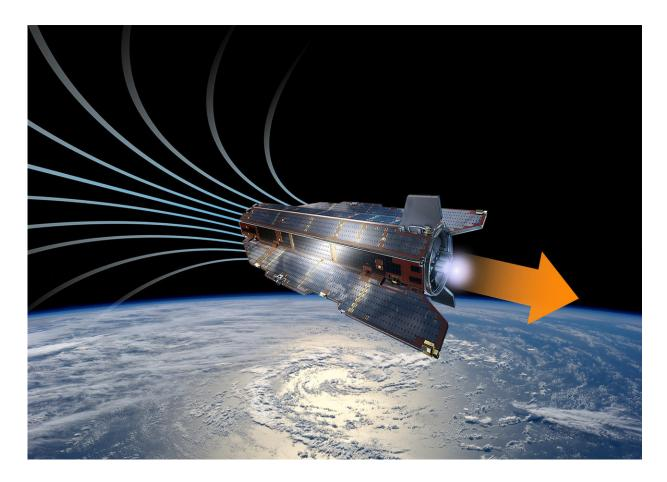
A future air-breathing space mission in low orbit around Earth: propelled at around 7.8 km/s, the satellite would ingest air molecules from the top of the atmosphere (left) to fire its ion thruster (right), providing thrust to overcome atmospheric drag, allowing it to stay in low orbit indefinitely. Credit: ESA–A. Di Giacomo
