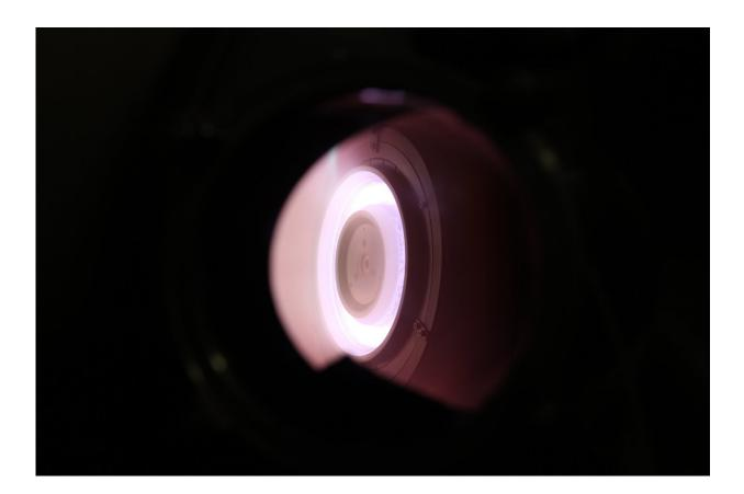
Fired at first using standard xenon propellant, the test thruster was then shifted to atmospheric air, proving the principle of air-breathing electric propulsion. Credit: ESA
