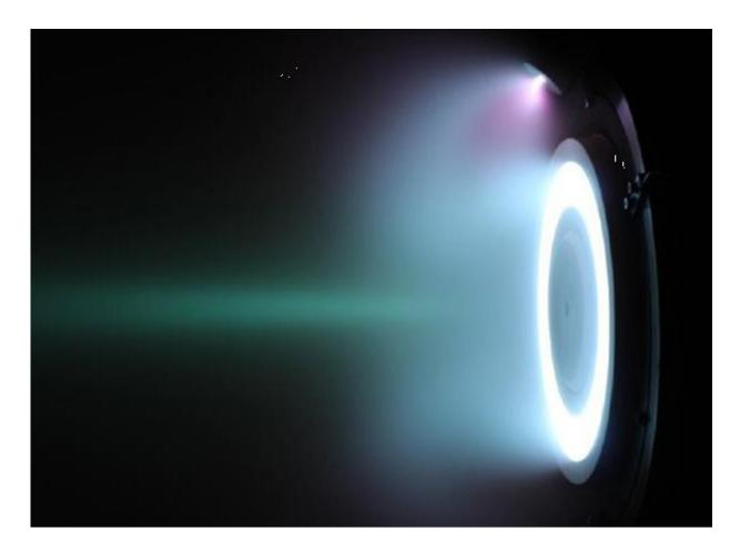
The air-breathing thruster was initially run with standard xenon propellant, causing a bluish plume, which was then progressively replaced with a mixture of nitrogen and oxygen to represent Earth's atmosphere. Success was marked by the thruster plume changing to purple. Credit: ESA/Sitael
