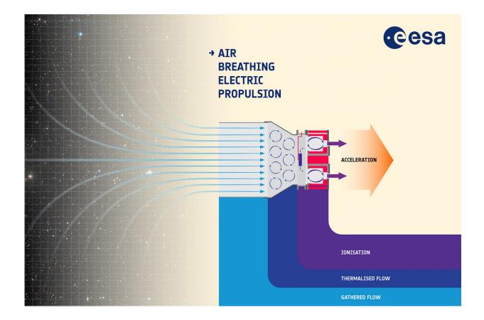
Molecules of air at the top of the atmosphere are captured by a novel type of intake, then collected and compressed to the point of becoming thermalised ionised plasma, at which point they can be given an electric charge to accelerate them and eject them to provide thrust. Air-breathing electric propulsion could make a new class of long-lived, low-orbiting missions feasible. Credit: ESA–A. Di Giacomo
