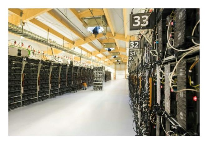
Souped-up computers called mining rigs operate 24/7, using huge amounts of electricity and generating lots of heat
