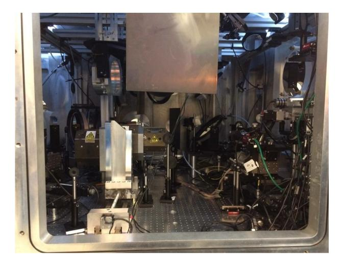
The target chamber, with optics used to focus the beams. Credit: Imperial College London
