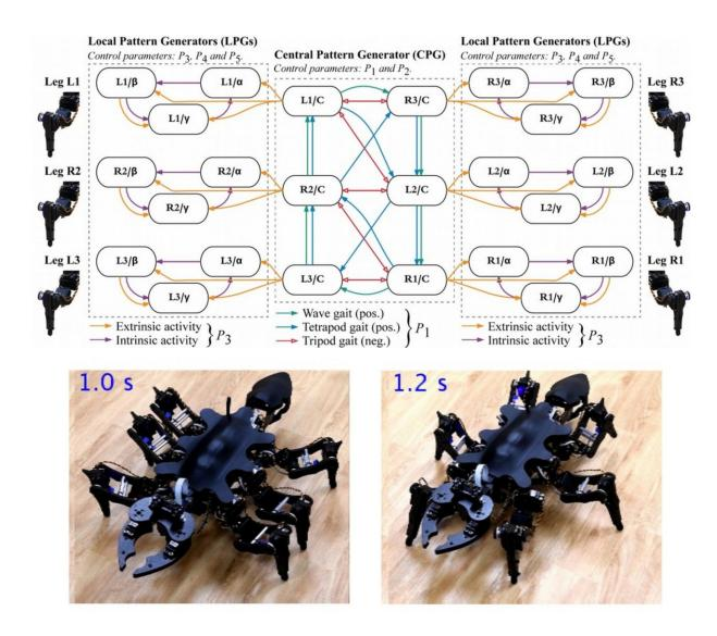
Top: Architecture of the controller, showing the central pattern generator, which controls the overall gait pattern, and at both sides, the six local pattern generators, which control individual leg trajectories. Bottom: Representative stillimages of the robot walking in an ant-like posture (left) and a cockroach-like posture (right). Credit: IEEE ACCESS
