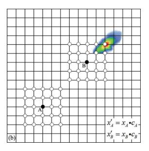
The perturbation is rescaled by the (a) traditional BGM method ?( b) LBGM method. (xA and xB are perturbations of A and B before rescaling; x'A and x'B are perturbations of A and B after rescaling; c is the scaling factor in the traditional BGM method; cA and cB are scaling factors of A and B in the LBGM method.) Credit: Science China Press
