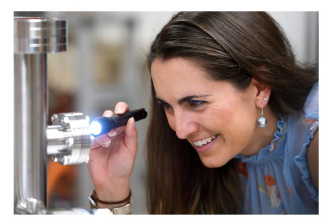
Hörst uses a flashlight to look inside the experimental chamber when the experiment is running, to see if haze is being formed. Credit: Will Kirk/JHU
