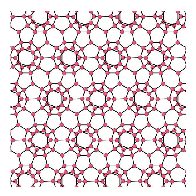
A clathrate ice, with oxygens represented as spheres, and hydrogen-bonds as
