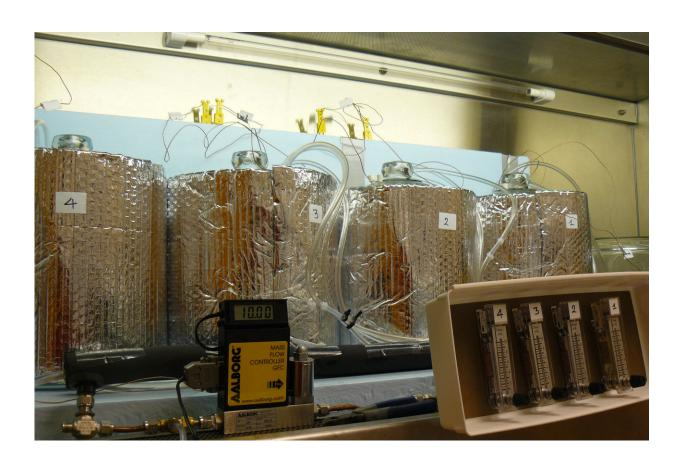
The researchers tested lab-scale aerobic digestion using tanks containing chicken carcasses, water and low levels of oxygen. Further research may test the concepts at field scale. Credit: Jacek Koziel
