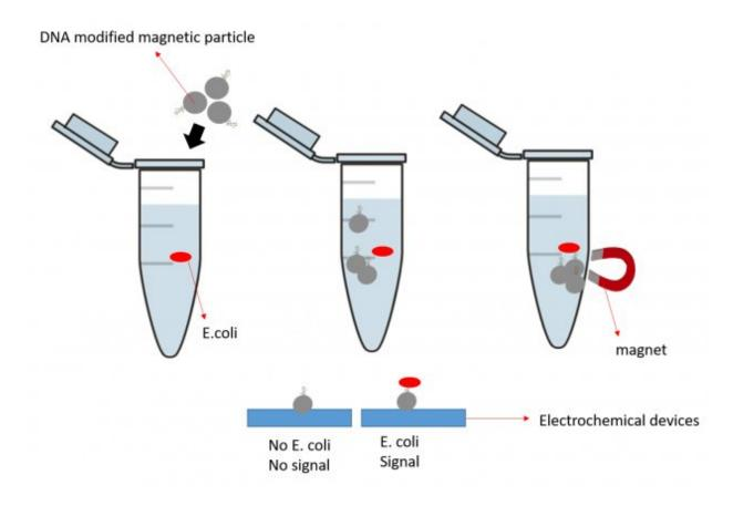
The sensor uses DNA-modified magnetic particles added to a water sample.
