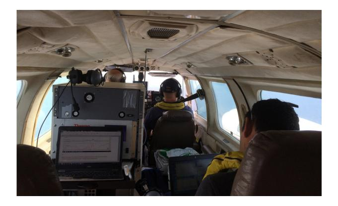
The inside of the sulphur-detecting plane. The sniffer is the big box on the left. Credit: Johan Mellqvist
