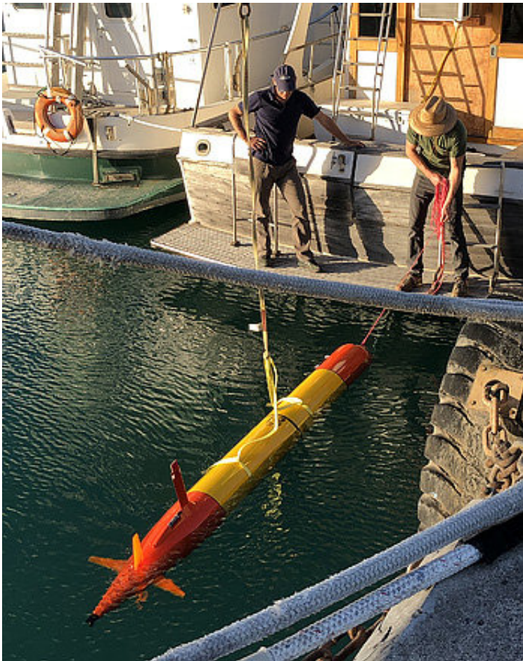
MBARI engineers Brett Hobson and Brian Kieft dunk-test the long-range AUV in Honolulu Harbor. Image: Chris Preston/MBARI
