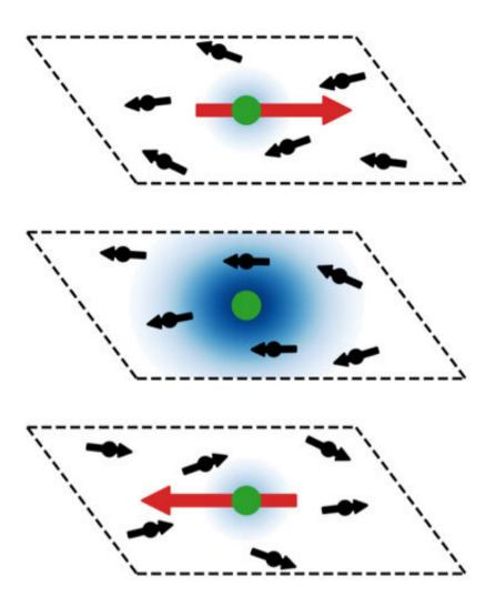
A graphic of a spontaneously emerging interface in a quantum material is shown. In the top and bottom layers the atoms (green dots) of the investigated material carry a magnetic moment (red arrow) that points in opposing directions. In these layers these magnetic moments are not correlated with the surrounding electrons
