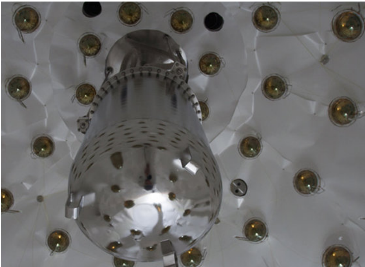
DarkSide-50 time projection chamber cryostat filled with liquid argon at Gran Sasso National Laboratory in Italy. Credit: DarkSide Collaboration
