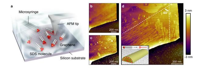
Images of experimental setup and AFM images. Credit: Nagoya University
