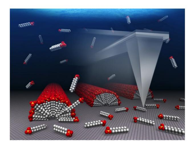
Molecular assemblies on graphene grow in perfect orientation by atomic force microscopy (AFM) tip scanning. Credit: Nagoya University
