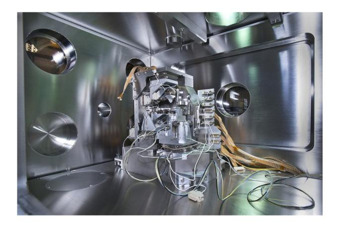
Researchers used this instrument to observe the nanowire defects discussed in this study. It is designed to deliver novel X-ray capabilities that bring researchers closer to the goal of observing materials at nanometer resolution. Credit: Brookhaven National Laboratory
