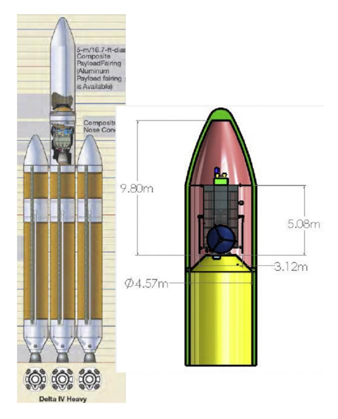
The 8.8-ton conceptual HAMMER spacecraft (right) is designed to fit within the Delta IV Heavy, the world's second highest-capacity launch vehicle in operation,
