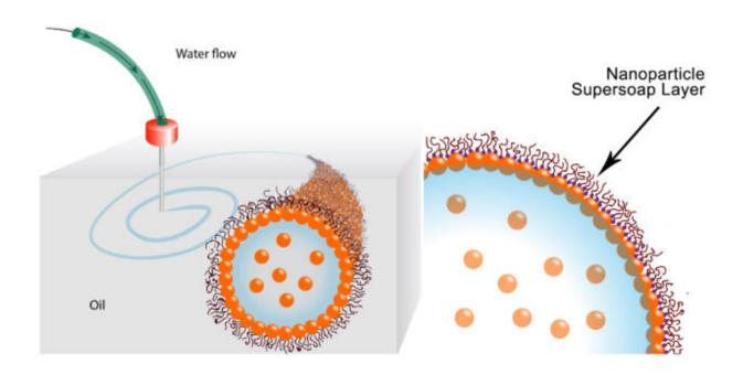
These schematics show the printing of water in oil using a nanoparticle supersoap. Gold nanoparticles in the water combine with polymer ligands in the oil to form an elastic film (nanoparticle supersoap) at the interface, locking the structure in place. Credit: Berkeley Lab
