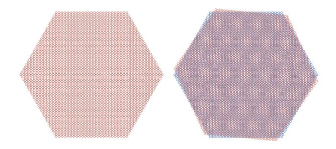
Physicists at MIT and Harvard University have found that graphene, a lacy, honeycomb-like sheet of carbon atoms, can behave at two electrical extremes: as an insulator, in which electrons are completely blocked from flowing; and as a superconductor, in which electrical current can stream through without resistance. Credit: MIT
