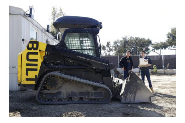
Bichen Wu, center, and Ed Walker use a laptop to determine what a autonomous bulldozer is seeing at Built Robotics Wednesday, Feb. 21, 2018, in San Francisco. Backed by Silicon Valley money, tech startups are developing selfdriving bulldozers, drones to inspect work sites and robot bricklayers that can lay bricks faster than human and work without lunch breaks. (AP Photo/Marcio Jose Sanchez)
