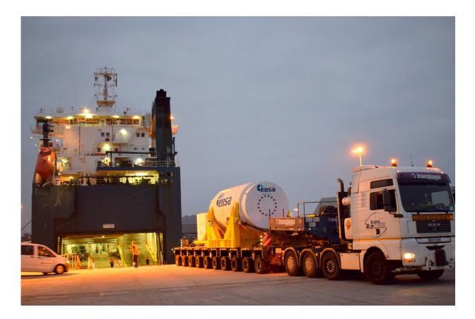
Loading the nuclear waste transportation and storage cask with three surrogate fuel rod assemblies onto a barge for the second leg of Sandia National Laboratories' triathlon. Credit: Sandia National Laboratories
