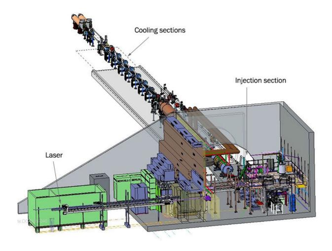
Schematic of low-energy electron cooling components. Credit: US Department of Energy
