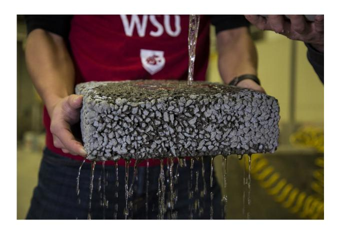
Water runs through Washington State University pervious pavement. Credit: Washington State University
