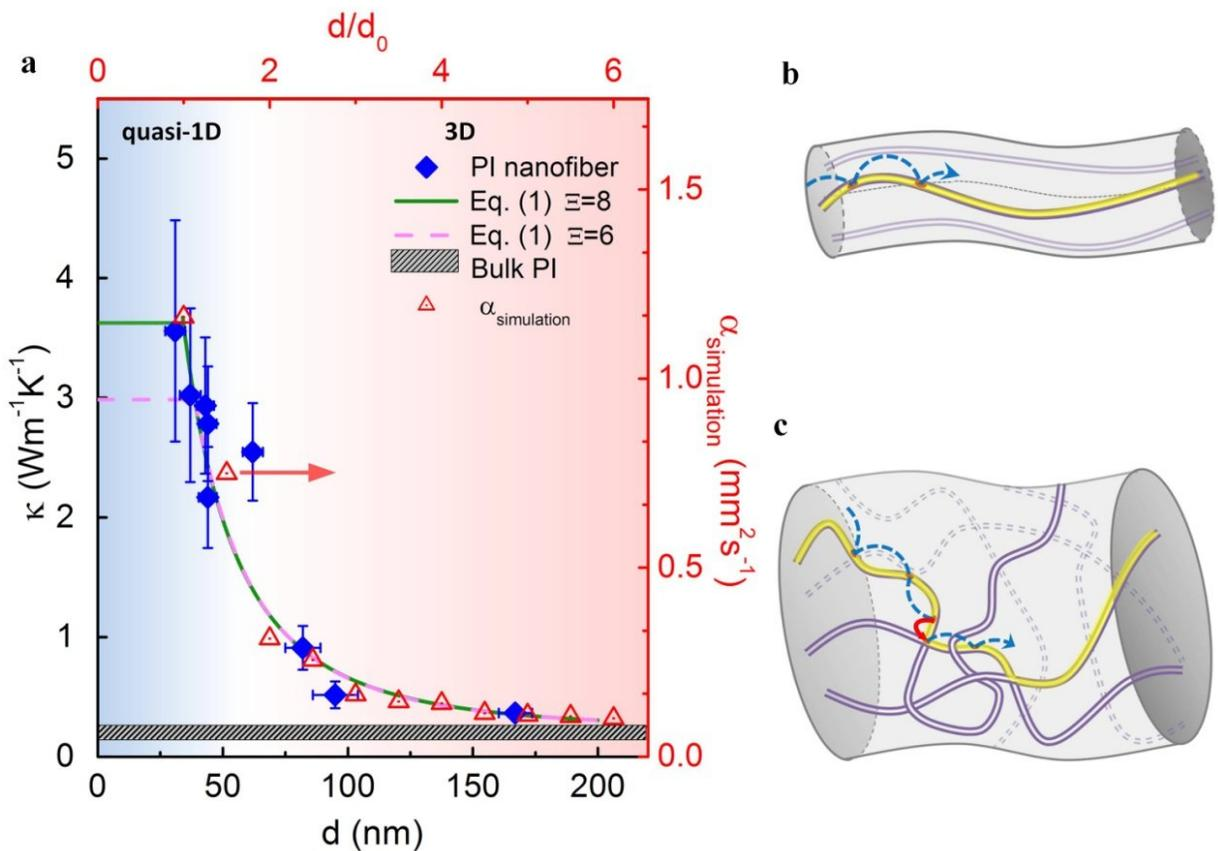
(a) The diameter dependence of the thermal conductivity of polyimide nanofibers. The rhombus represents experiment data. There is a dimensional crossover of heat diffusion in molecular chains from quasi-1D to 3D. (b) Schematic of anisotropic quasi-1D thermal diffusion in nanofibers with small diameters. All the molecular chains are aligned along the fiber axis. The blue arrow denotes the 'random walk' of heat carriers within the chain. (c) Schematic
