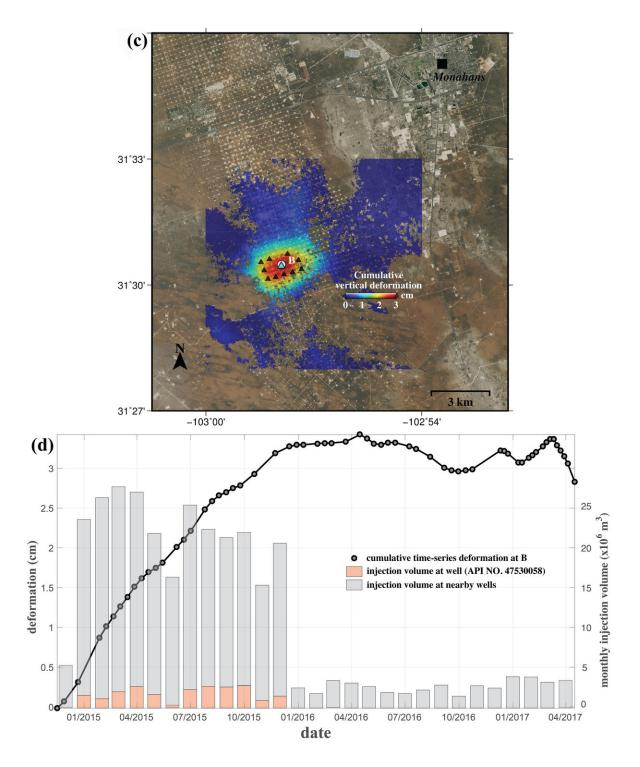
In the vicinity of 11 carbon dioxide (CO2) injection wells nearly seven miles southwest of Monahans, Texas, the radar analysis detected surface uplift of more than 1 inch. As with wastewater injection, CO2 injection increased pore pressure in the rocks, so when stress was relieved it was followed by uplift. (Zhong Lu
