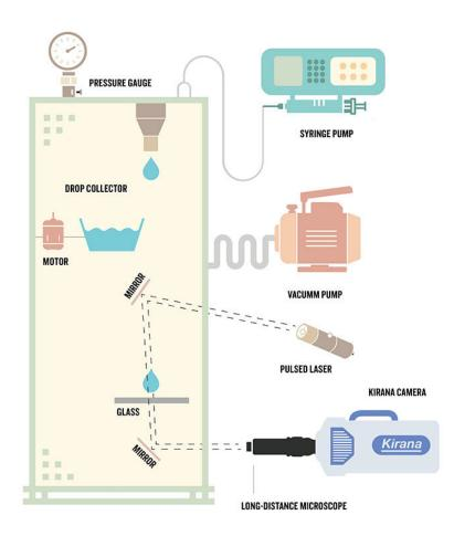
Sigurdur Thoroddsen and his team from KAUST set up an experiment to test whether bubble formation would be suppressed at lower air pressures. The team created a vacuum chamber equipped with a high-speed camera to observe droplet bubble formation. Credit: King Abdullah University of Science and Technology
