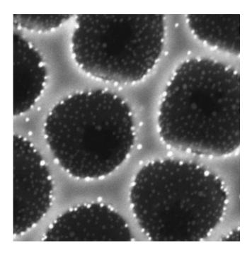
The researchers introduced a co-assembly method in which tiny, spherical particles and matrix precursors are deposited simultaneously from a single mixture to produce defect-free films over centimeter scales. The researchers demonstrated this process with widely-used catalytic materials, including titania, alumina and zirconia, incorporating various mono and multi-metallic nanoparticles. Credit: Harvard University
