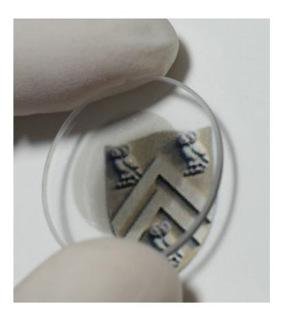
A wafer of highly aligned carbon nanotubes, seen in gray on a piece of glass, facilitated a novel quantum effect in experiments at Rice University. Credit: Jeff Fitlow
