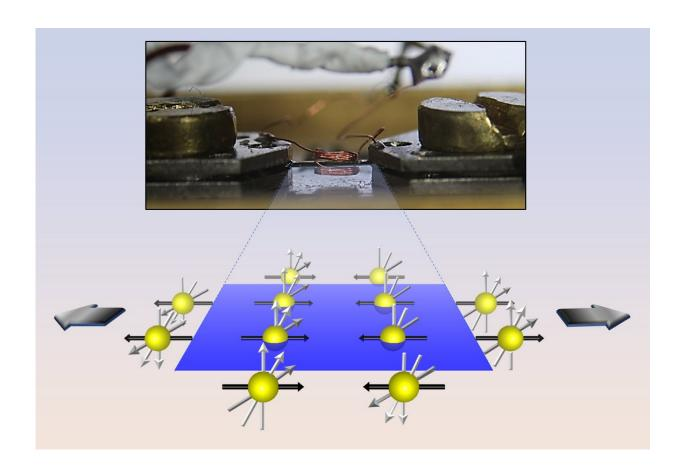
Top: A piece of BaFe2As2 is stretched while magnetic measurements are taken (the copper wire coil is part of the NMR device). Lower diagram shows atoms in a plane, with black arrows showing how magnetic spins lie in plane and point in opposite directions. Grey arrows show how the magnetic spin of atoms shifts as the material is stretched. Credit: Nicholas Curro, UC Davis
