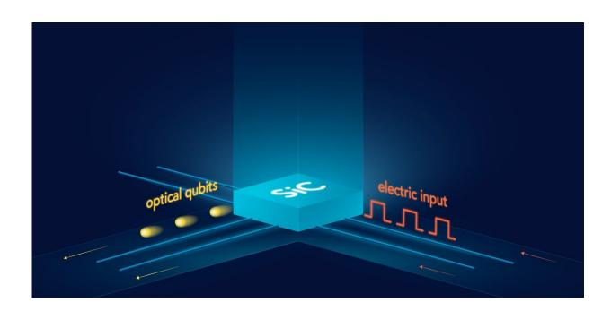
Electrical excitation causes a point defect in the crystal lattice of silicon carbide to emit single photons, which are of use to quantum cryptography. Credit: Elena Khavina, MIPT
