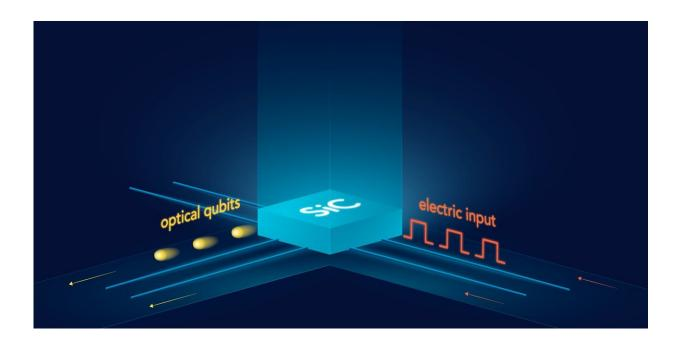
Electrical excitation causes a point defect in the crystal lattice of silicon carbide to emit single photons, which are of use to quantum cryptography. Credit: Elena Khavina, MIPT
