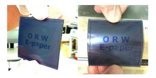
Combined flexible blue optically rewritable LCD. Credit: Zhang et al.
