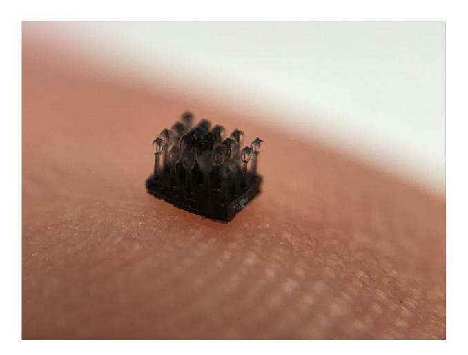
For years, scientists have been inspired by nature to innovate solutions to tricky problems, even oil spills -- manmade disasters with devastating environmental and economic consequences. A new USC study takes a cue from leaf structure to fabricate material that can separate oil and water, which could lead to safer and more efficient oil spill clean-up methods. Credit: Yang Yang
