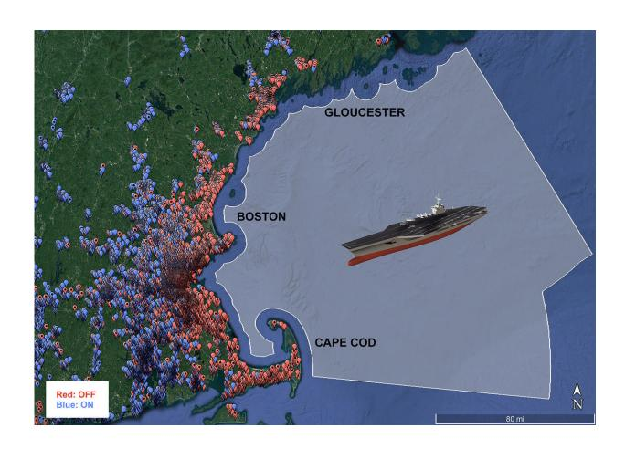
NIST simulation showing wireless users of shared radiofrequency (RF) spectrum in the Boston to Cape Cod, Massachusetts, region. Colored markers identify users that can continue operating (blue) or must be shut off (red) to accommodate priority need for wireless band by naval vessel within offshore "designated protection area" (gray). Credit: Michael Souryal/NIST (using Google Earth map of Massachusetts coast)
