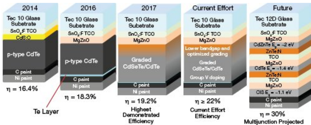
Figure 1. Researchers at Colorado State Univ. have created a roadmap of device structures for CdTe PV performance. Thus far, they have achieved efficiencies of 19.2%. Credit: Colorado State University
