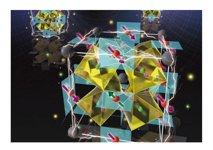
A newly discovered material called BiMn3Cr4O12, represented by the crystal structure, exhibits a rare combination of magnetic and electrical properties. The arrows illustrate the spin moments for the elements chromium (Cr) in yellow and manganese (Mn) in blue. Studying this material's behavior could lead to improved applications in technology and information storage. Credit: Institute of Physics, Chinese Academy of Sciences/Youwen Long
