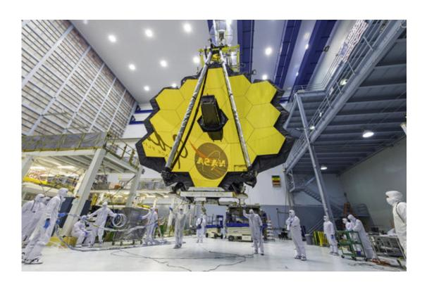
In this April 13, 2017 photo provided by NASA, technicians lift the mirror of the James Webb Space Telescope using a crane at the Goddard Space Flight Center in Greenbelt, Md. The telescope's 18-segmented gold mirror is specially designed to capture infrared light from the first galaxies that formed in the early universe. On Tuesday, March 27, 2018, NASA announced it has delayed the launch of the next-generation space telescope until 2020. (Laura Betz/NASA via AP)
