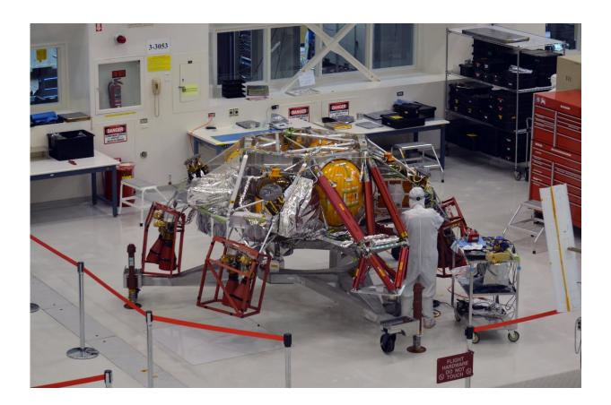
A technician works on the descent stage for NASA's Mars 2020 mission inside JPL's Spacecraft Assembly Facility. Mars 2020 is slated to carry NASA's next Mars rover to the Red Planet in July of 2020. Credit: NASA/JPL-Caltech
