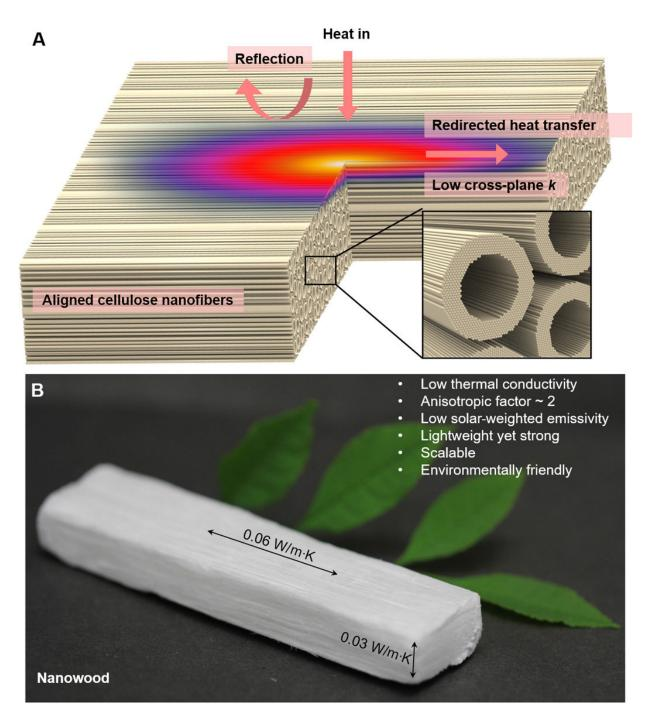
Completely derived from natural wood, nanowood with hierarchically aligned cellulose nanofibrils can be used as an anisotropic super thermal insulator. (A) Schematics of the thermally insulating properties of the nanowood. (B) Digital photograph of the nanowood and the corresponding properties beneficial for building insulation applications. Credit: *Science Advances* (2018). DOI: 10.1126/sciadv.aar3724
