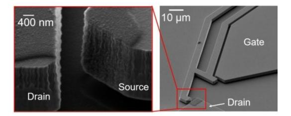
A microelectromechanical relay with the contact electrode surfaces covered by a 100nm thick layer of nanocrystalline graphite (inset). Credit: University of Bristol
