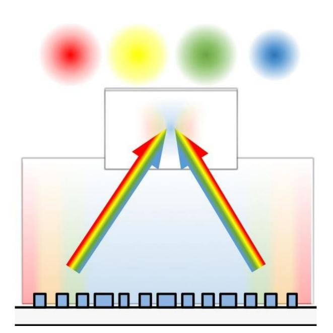
Schematic of multiwavelength achromatic metalens. In addition to acting as a beam and hologram generator, this metalens can also focus four different wavelengths of light (R, Y, G, and B) at the same distance. Credit: Capasso
