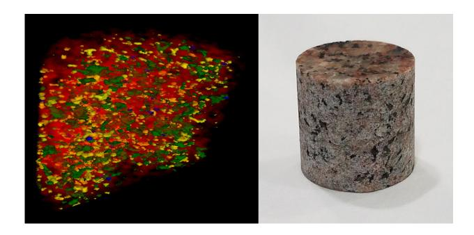
The neutron interferometer can scan the interior of thick objects, such as this chunk of granite, providing enough detail to show the four types of rock that are mixed within it. Credit: Huber & Hanacek, NIST
